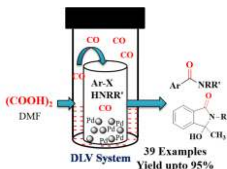
Fig. 1 Pd@PS catalyzed cyclic and non-cyclic amides synthesis
