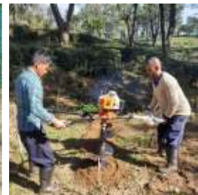
One man earth auger method Two men earth auger method
