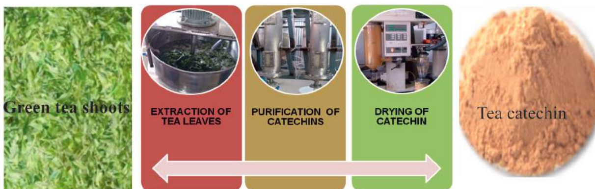
Fig. 3 Process up-scaled up to 40 kg per batch green tea leaves processing
